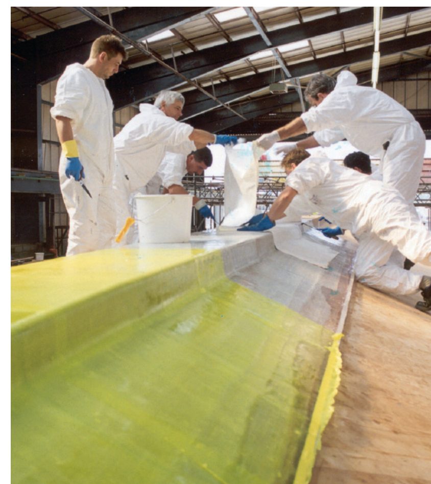
Hull sheathing for Tenacious, the world's largest wooden tall ship
