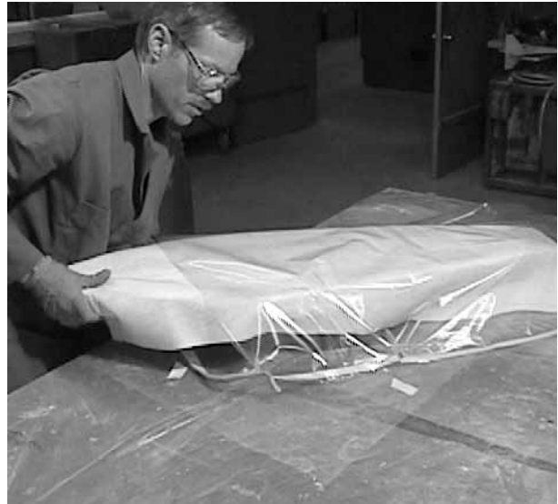
10. Place the mold and lay-up inside a vacuum bag envelope. Make the envelope by folding a large sheet of plastic in two and sealing the three open sides with mastic. Seal two sides of the envelope before beginning the lay-up. Peel the protective paper from the mastic and seal the third side after the mold is placed inside.
