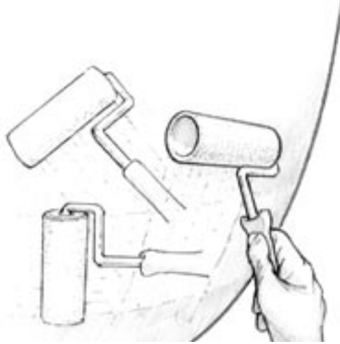
Figure 3-19 Apply the epoxy in thin even coats with a thin foam roller.
