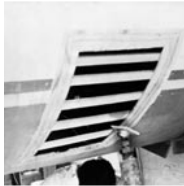
Figure 6-16 Bevel the edges and fasten temporary stringers to the back of the opening.
