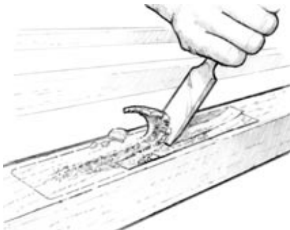
Figure 4-1 Use a chisel to excavate a cavity that extends beyond all of the damaged wood.
